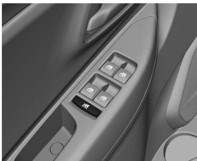
Pulse el interruptor
